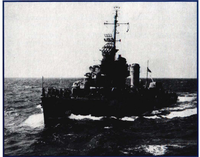
The USS Aaron Ward, a Benson-class destroyer, photographed on 17 August 1942. Note the gun director turret with radar antenna above the bridge. (National Archives.)
